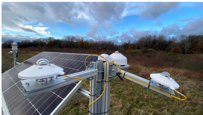
Autonomous measurement station on site. Pyranometers in several orientations, with temperature, humidity and microclimatic variables, recorded every five minutes.
