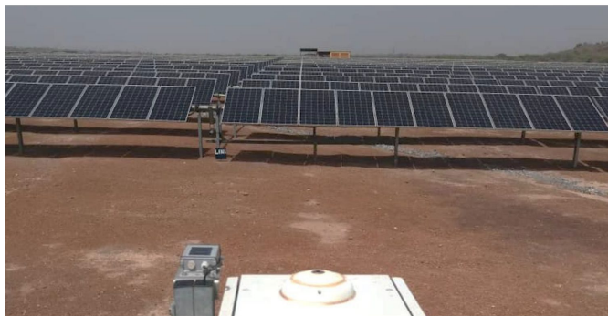
Measurement station and PV field at Loulo. Hemispherical fisheye cameras placed around the plant capture cloud formations that satellite imagery and irradiance sensors do not resolve.
