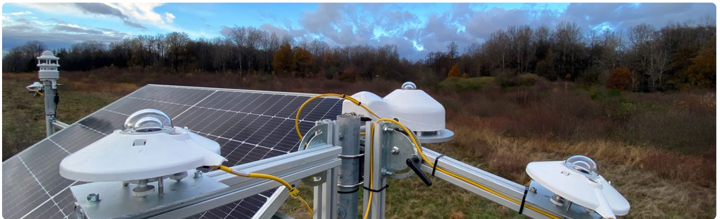
Autonomous measurement station on a client site. Irradiation in several orientations, temperature, humidity and key microclimatic variables, recorded at 5-minute intervals over a full 12-month cycle.
